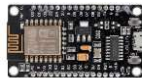
Gambar 2.2 NodeMCU ESP8266 Sumber: (Solemede, Haidar, & Rahayu, 2020)
