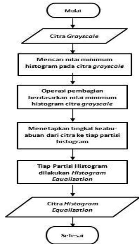
Gambar 8. Diagram Alir Histogram Equalization
