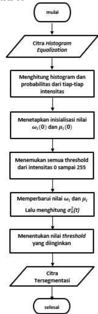
Gambar 10. Diagram Alir Otsu's Thresholding
