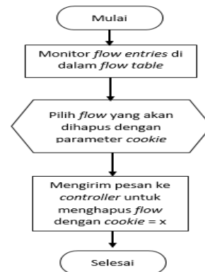
Gambar 1. Mekanisme Idle Timeouts
