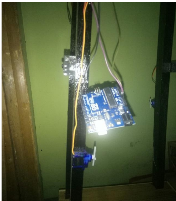
Gambar 5. Implementasi Servo Motor.
