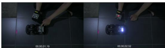
Gambar 15. Pengujian Delay Response Time Awal
