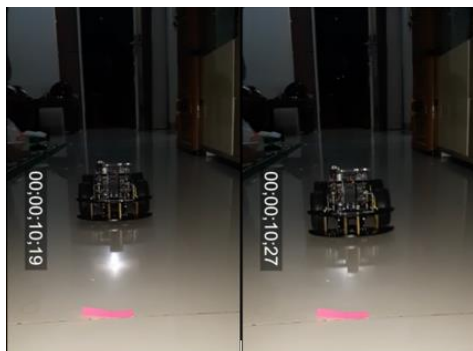
Gambar 14. Pengujian Delay Response Time Jarak 10 Meter
